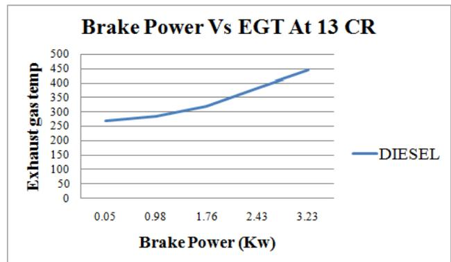
Fig. 5. Brake Power Vs EGT for Diesel
