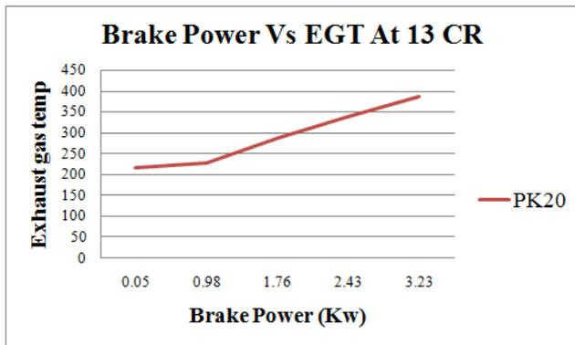
Fig. 6. Brake Power Vs EGT for PK20
