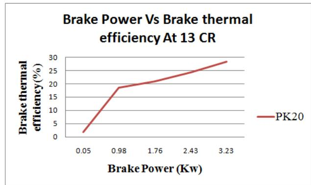
Fig. 2. Brake Power Vs Brake thermal efficiency for PK20
