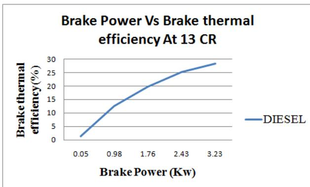
Fig. 1. Brake Power Vs Brake thermal efficiency for diesel
