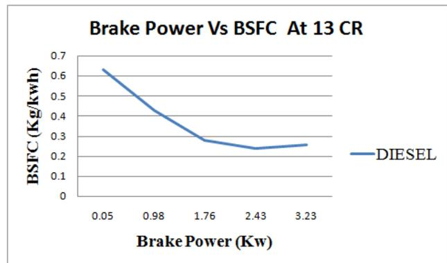
Fig. 3. Brake Power Vs BSFC for Diesel
