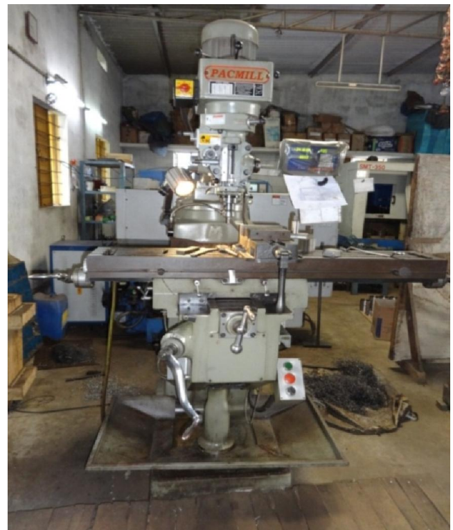
Fig 1. Vertical milling machine (PAC mills)
