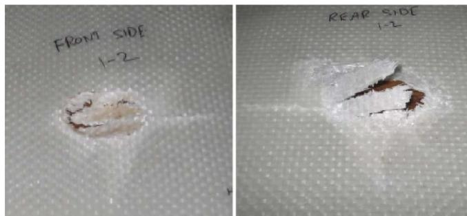
Figure 7. Damage pattern of laminate 1-2 under bullet impact
