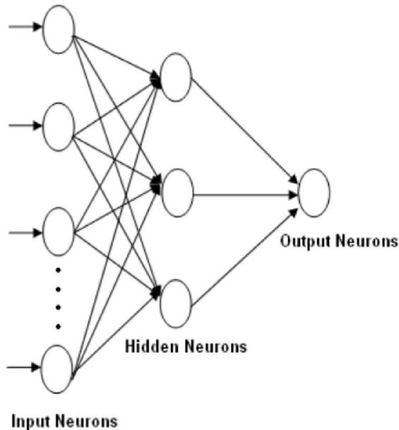
Figure 7. Architecture of Feed Forward Neural Network
