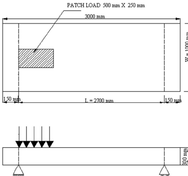
Fig. 3. Position of patch load at support of GFRP bridge deck panel
