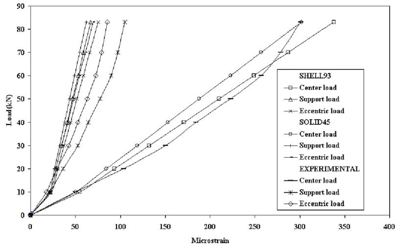
Fig. 14. Load vs strain at midspan of GFRP bridge deck panel
