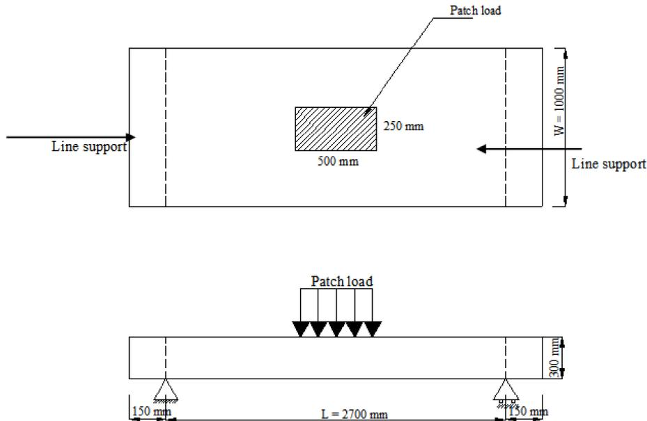
Fig. 2. Position of patch load at center of GFRP bridge deck panel
