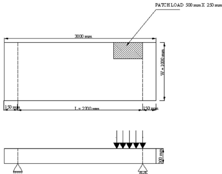
Fig. 4. Position of patch load at corner of GFRP bridge deck panel
