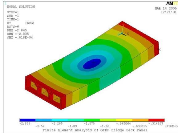
Fig. 8. Deflection contour of GFRP bridge deck panel using SOLID45 element
