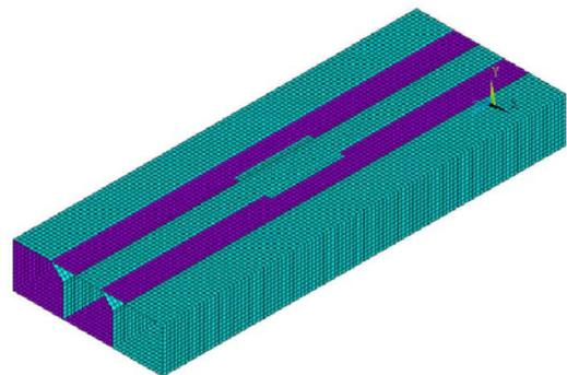
Fig. 6. Discretization of GFRP bridge deck panel using SHELL93 elements
