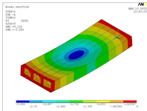
Fig. 10. Deflection contour of GFRP bridge deck panel using SHELL93 element
