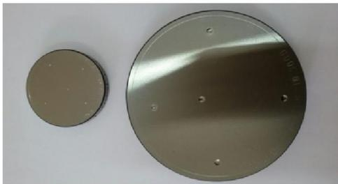
**Figure 3. Hardness tested blocks, Block 1<sup>st</sup> (2.5/187.5) (left), Block 2<sup>nd</sup> (10/3000) (right). {Ref: NPL}**
