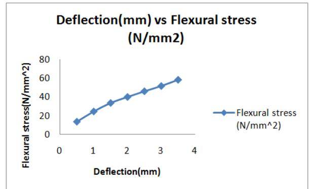
**Graph 2. Mean values of flexure stress by deflection for fiber 6mm untreated composite**
