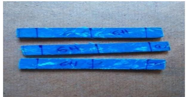
Fig.9. Flexural Test Specimens
