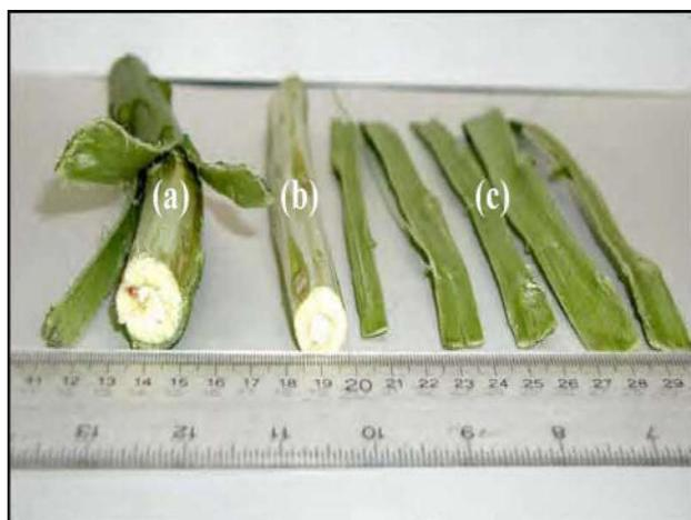
Fig.2. Kenaf Bast and Core parts
