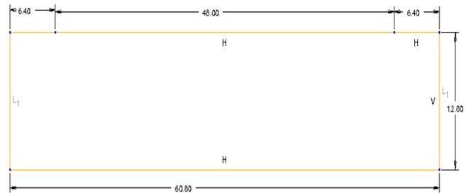
Fig.8. ASTM – D790 Flexural Test Specimen
