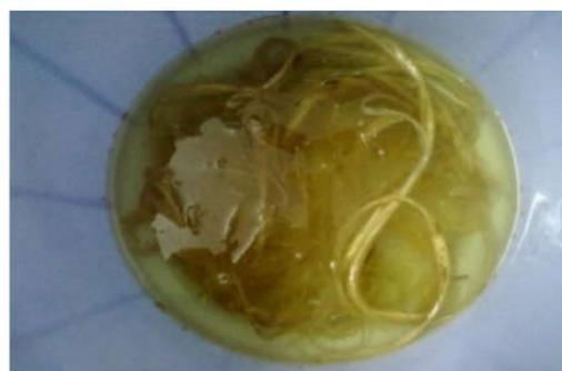
Fig.3 Treatment of Fiber in 2% NaOH solution
