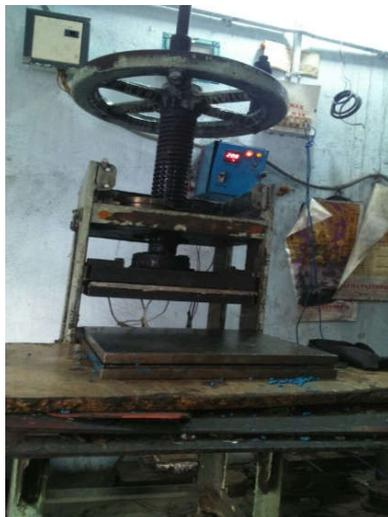
Fig.7. Compression moulding machine setup
