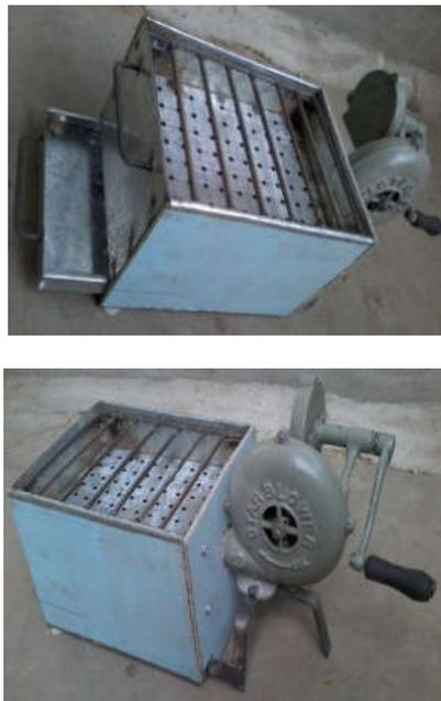
**Fig. 1. The Improved Barbecue Stove:** It was designed with features to minimize the stress on arms, probability of accidents and improving the performance of the stove. The stove is in cubical shape with insulations to avoid the direct contact of heat to the body and the provisions were made to avoid the contact of fire with the body part (fingers). Instead of making use of hand fan, a blower was attached to the model to reduce the stress produced by constant fanning
