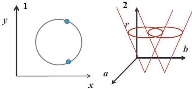
Figure 4. Find Circle parameters if radius were unknown. 1- original space, 2- parametric space
