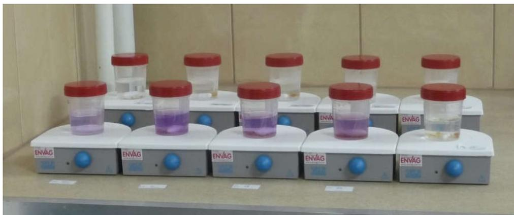
Figure 7. Mixtures of chitosan hydrogels and heavy metal ions solutions
