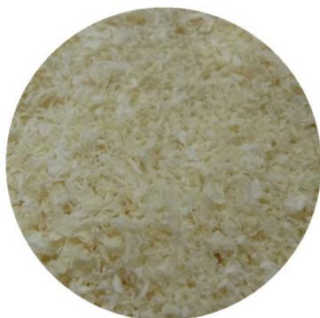
**Figure 2. Commercial sample of chitosan flakes produced by Vanson company (Deacetylation Degree 74%)**
