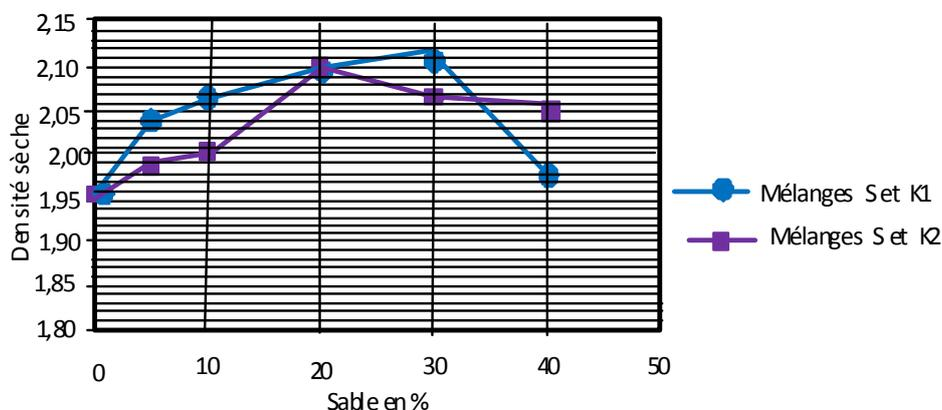
Figure 6. Dry density for Modified Optimum Proctor for compounds according to percentage of sand added
