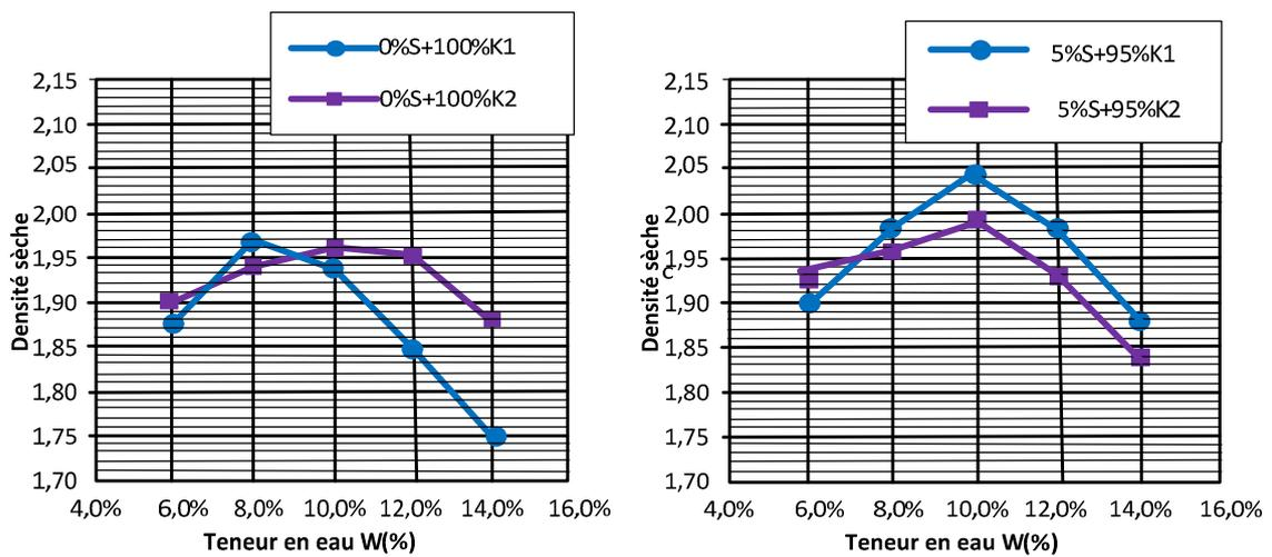
Figure 3. Densities according to water content for 0%S+100% (K1 or K2), 5%S+95% (K1 or K2) compounds
