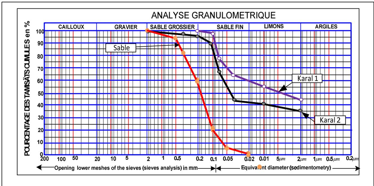
Figure 2. Résultats de granulométriques tests analyses of samples of Sanaga sand (sand) and swelling clay from Maroua (Kara1 or K1) and Fotokol (Kara2 or K2)
