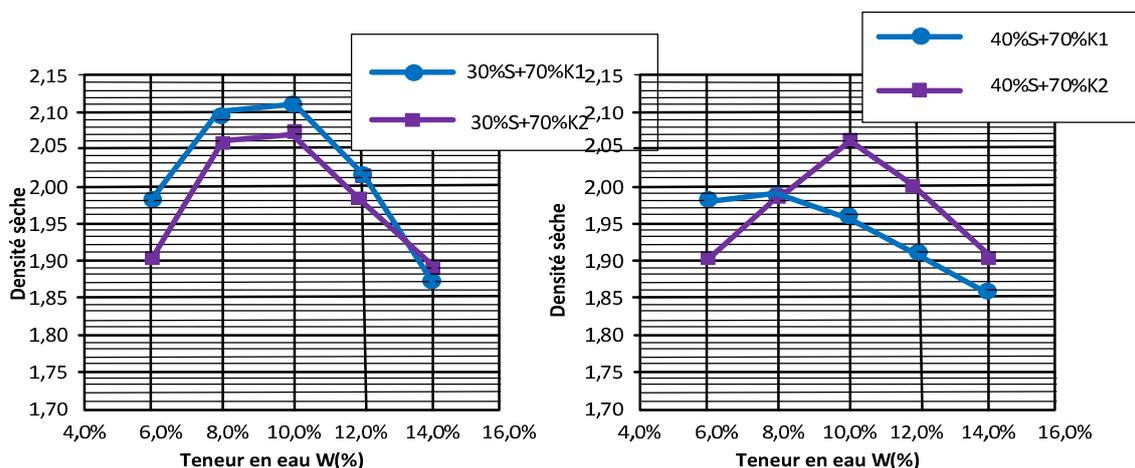
Figure 5. Densities according to water content for 30%S+70% (K1 or K2), 0%S+60% (K1 or K2) compounds
