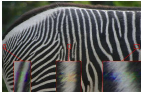
Figure 12. The edge misalignment increases with distance from the optical axis
