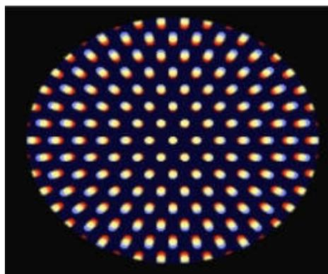
Figure 6. Lateral chromatic aberration (LCA)
