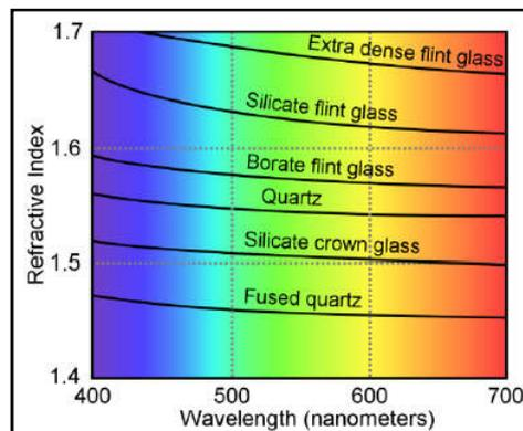
Figure 9. The variation of the refractive index of glass with wavelength
