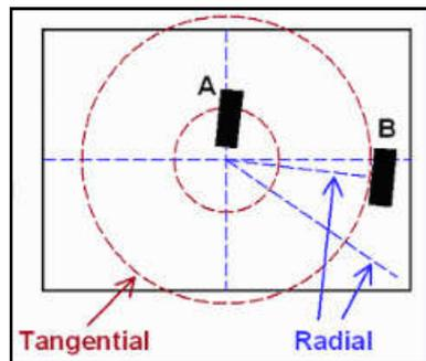
Figure 16. Measuring lateral Chromatic aberration using tangential edges
