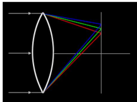
Figure 3. Lateral or transverse chromatic aberration (LCA). Magnification varies with color wavelength
