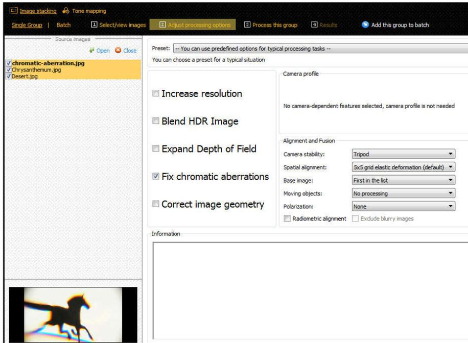
Figure 15. Fixing Chromatic Aberration by PhotoAcute
