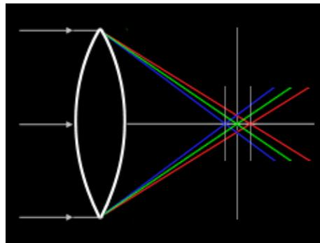
Figure 2. Axial or longitudinal chromatic aberration (ACA). Focal length varies with color wavelength
