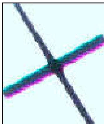
Figure 7. Lateral chromatic aberration (LCA)
