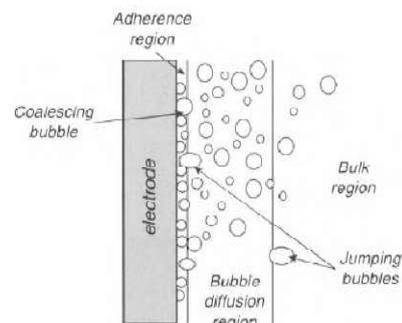
Figure 2. Bubble diffusion region of ECDM process
