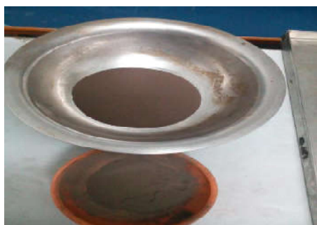
Figure 3. Top Container- Kansya Bhasma prepared by Muffle Furnace Bottom - Kansya Bhasma prepared by Puta
