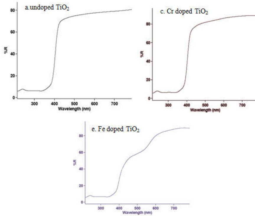
Fig. 2. Diffuse absorption spectra of undoped and metal ions doped  $\text{TiO}_2$
