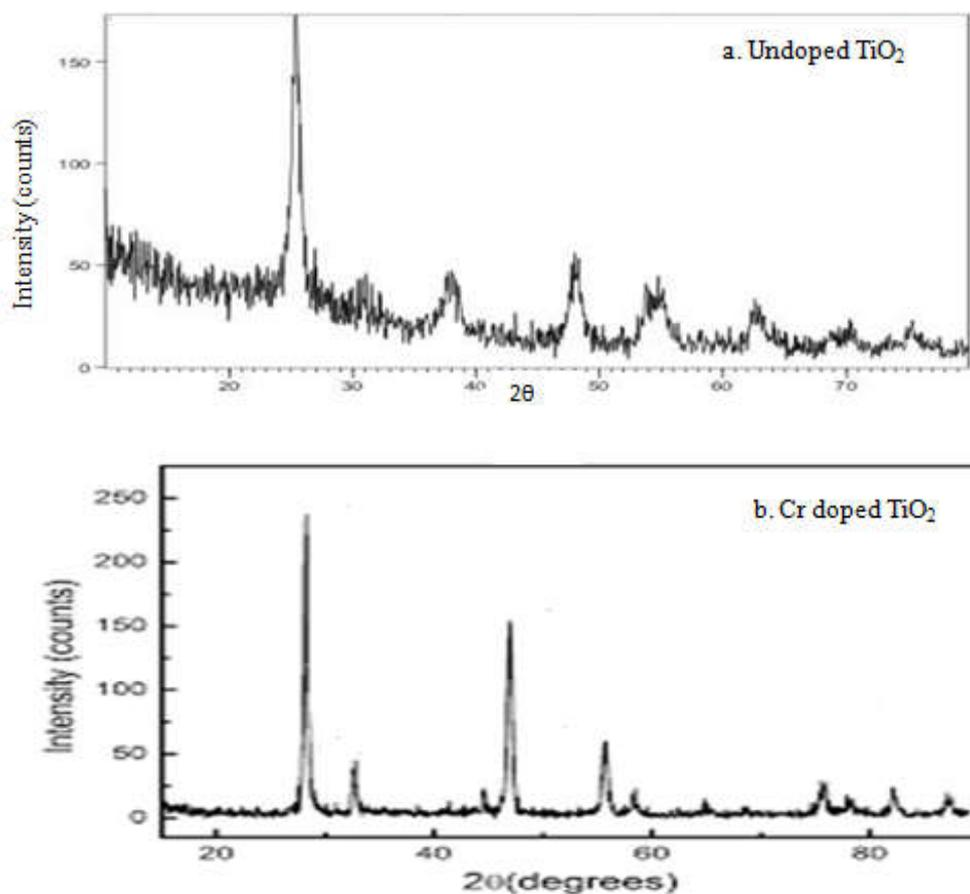
Fig. 4. X-ray diffractogram of undoped and Cr doped  $\text{TiO}_2$
