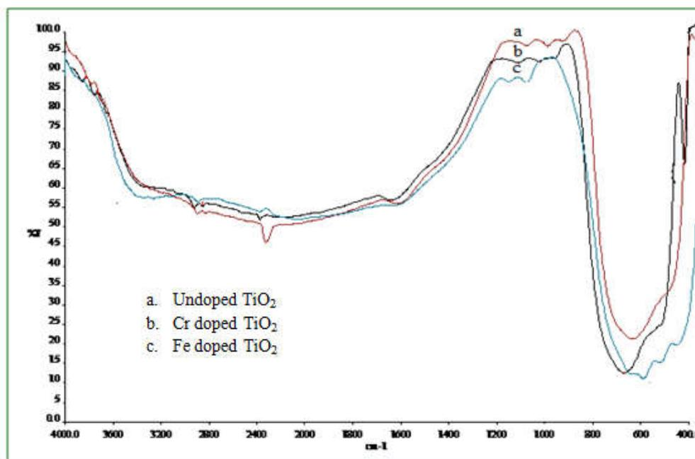
Fig. 1 IR Spectra of undoped and metal ions  $\text{TiO}_2$
