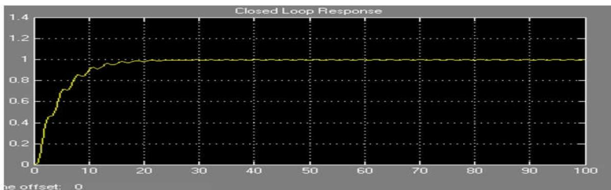
Figure 6. Simulated results PID controller of DC motor
