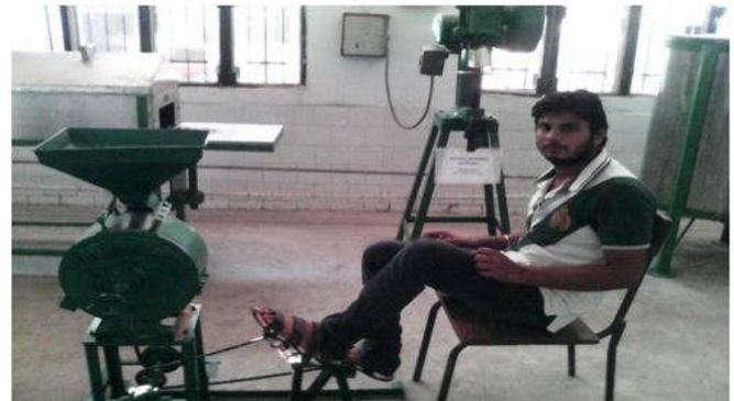
Figure 3. Pedal Operated Flour Machine
