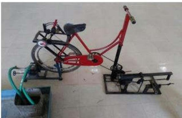
The machine comprise of various linkages, sprocket, chain drive mechanism and pedal assembly on which force is applied by an operator which indirectly convert the pedaling power into working stroke of hacksaw, which is 60 stroke/min and can cut 30mm diameter work piece of various materials like wood, PVC, plywood, hollow metal pipes and bars. Also the water pump can lift up the water from 10m to 16m by attaining speed up to 1890 to 1900 RPM. The DC motor can generate 12 v of
