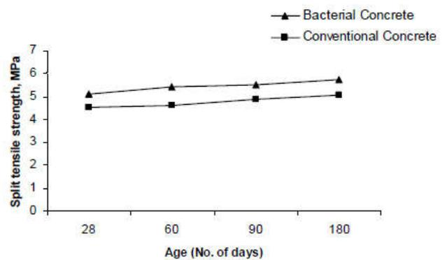
Fig.10. Variation of split tensile strength with age
