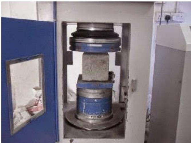
Fig.7. Test of Compressive Strength
