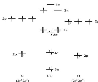
Figure 1. Molecular orbital energy level diagram for NO<sup>[4]</sup>
