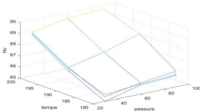
Figure 5. Hardness – Compounding Temperature-Compression Pressure ByMATLAB Enumeration method
