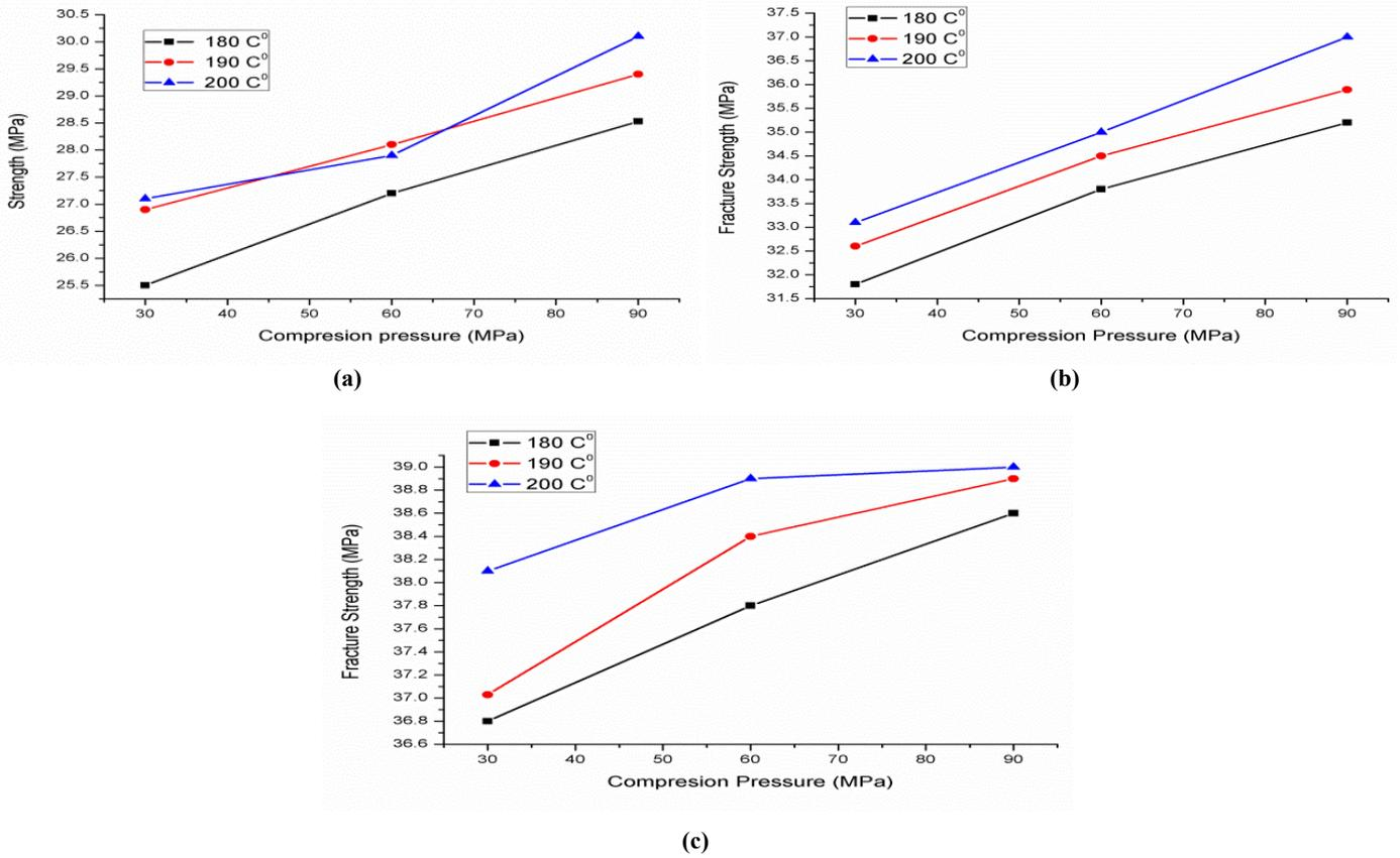
Figure 1. Relationship between compression pressure and fracture strength a) at 10 CaCO<sub>3</sub> /90PP, b) 20CaCO<sub>3</sub> /80PP, c)5Al<sub>2</sub>O<sub>3</sub>/20 CaCO<sub>3</sub> /75PP
