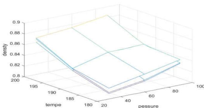
Figure 4. Density – Compounding Temperature-Compression Pressure ByMATLAB Enumeration method
