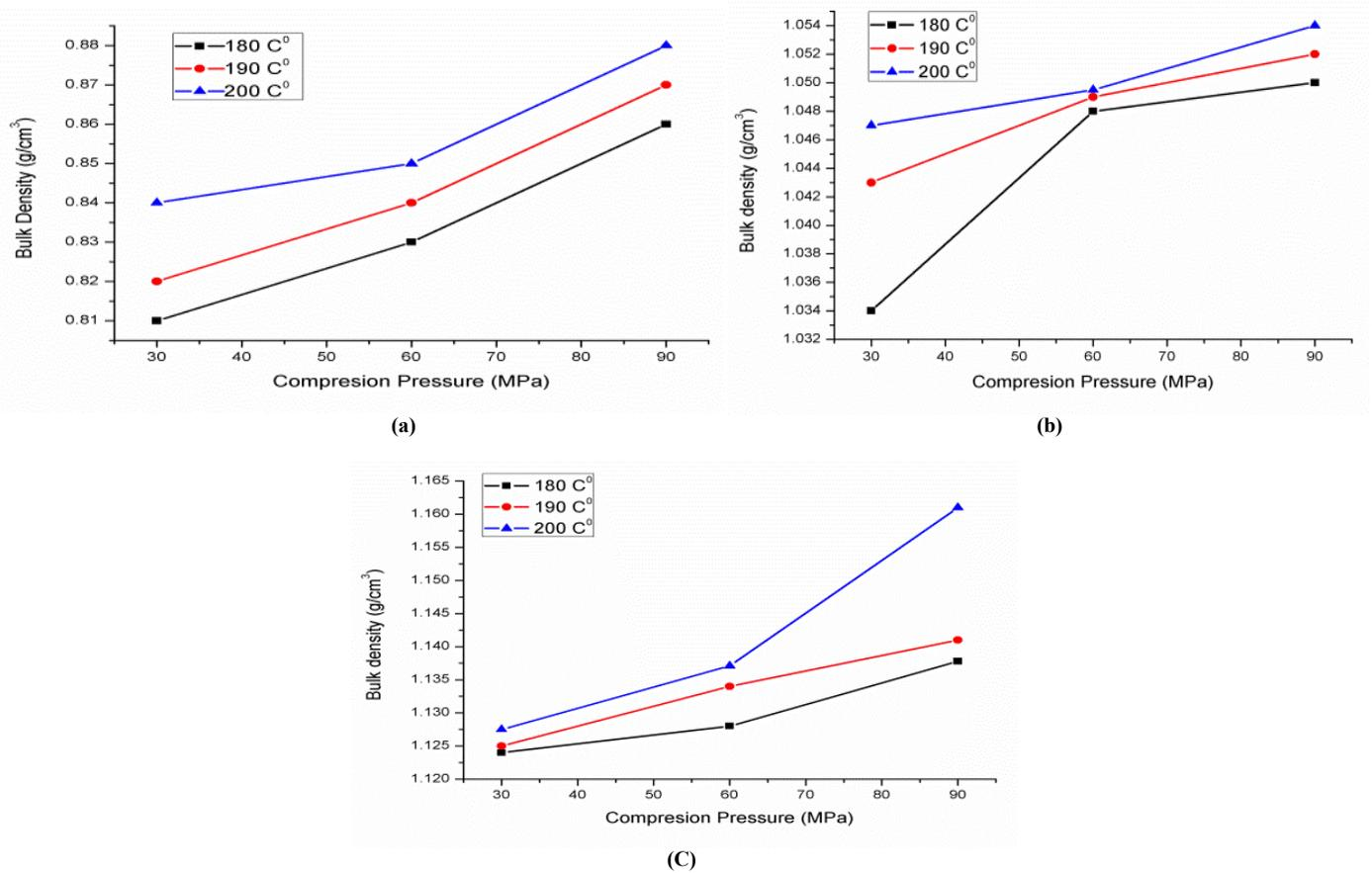
Figure 2. Relationship between compression pressure and Density a) at 10 CaCO<sub>3</sub> /90PP, b) 20 CaCO<sub>3</sub> /80PP, c) 5Al<sub>2</sub>O<sub>3</sub>/20 CaCO<sub>3</sub> /75PP
