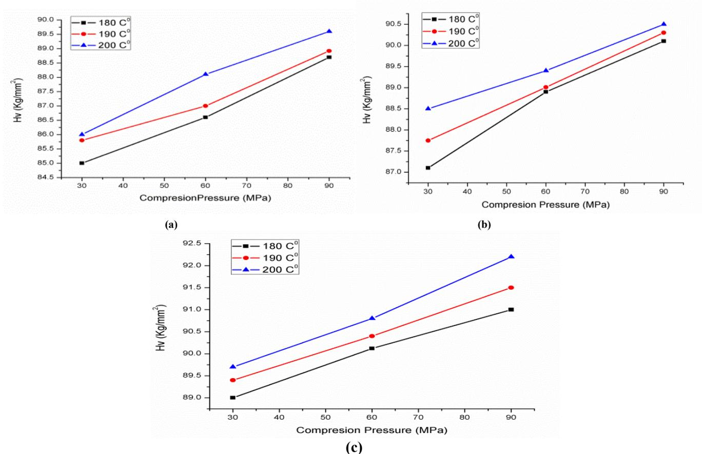
Figure 3. Relationship between compression pressure and microhardness a) at 10 CaCO<sub>3</sub> /90PP, b) 20 CaCO<sub>3</sub> /80PP, c) 5Al<sub>2</sub>O<sub>3</sub>/20 CaCO<sub>3</sub> /75PP
