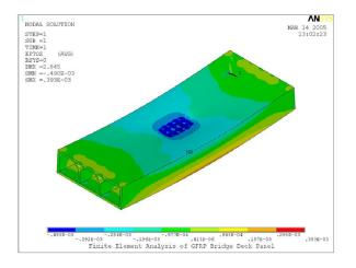
Fig. 9. Strain contour of GFRP bridge deck panel using SOLID45 element
