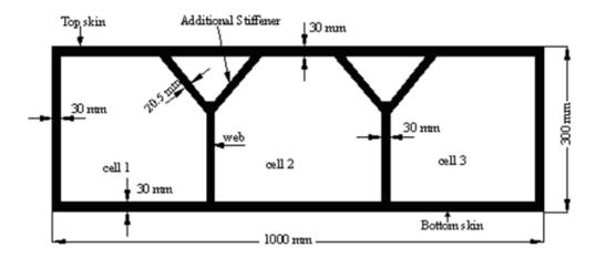
Fig. 1. Cross section of GFRP bridge deck panel
