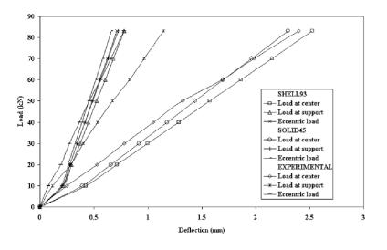
Fig. 12. Load vs deflection at midspan of GFRP bridge deck panel
