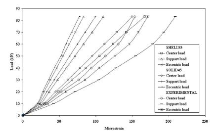
Fig. 15. Load vs strain at quarterspan of GFRP bridge deck panel
