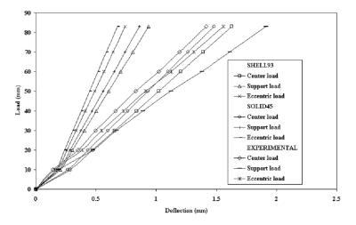
Fig. 13. Load vs deflection at quarterspan of GFRP bridge deck panel
