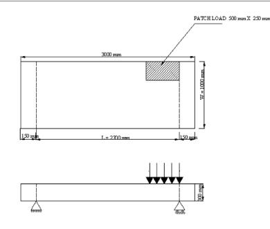
Fig. 4. Position of patch load at corner of GFRP bridge deck panel
