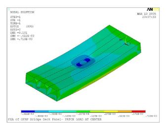
Fig. 11. Strain contour of GFRP bridge deck panel using SHELL93 element
