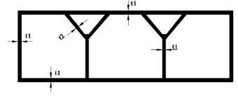
Fig. 7. Cross section of GFRP bridge deck panel in terms of parameters
