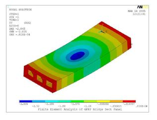
Fig. 8. Deflection contour of GFRP bridge deck panel using SOLID45 element
