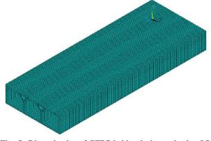
Fig. 5. Discretization of GFRP bridge deck panel using SOLID45 elements
