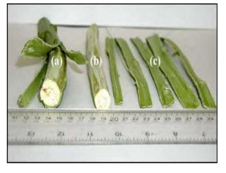
Fig.2. Kenaf Bast and Core parts
