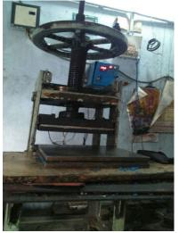
Fig.7. Compression moulding machine setup
