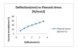
Graph 2. Mean values of flexure stress by deflection for fiber 6mm untreated composite
