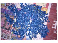
Fig. 5. Polypropylene pallets
