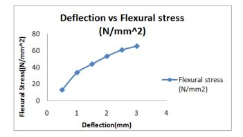
Graph 1. Mean values of flexure stress by deflection for fiber 6mm treated composite
