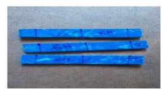
Fig.9. Flexural Test Specimens
