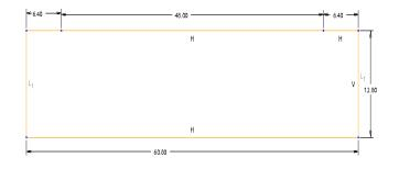
Fig.8. ASTM - D790 Flexural Test Specimen
