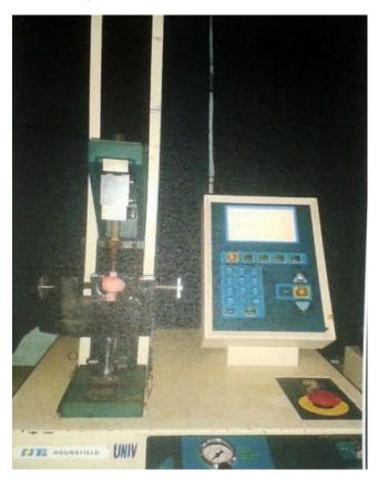
Fig. 4B. utm machine with specimen
