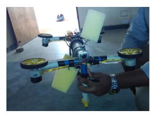
Figure 1. Developed Pipe Cleaning Robot
