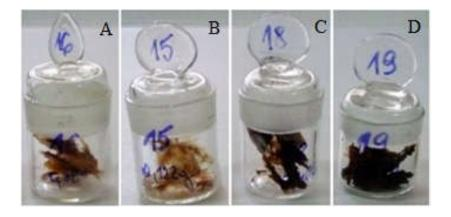
Figure 4. Dried hydrogel samples (Samples A, B, C, D)
