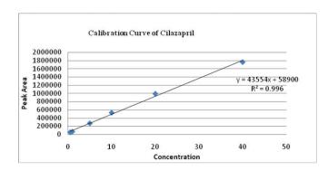
Fig. 10. Calibration curve of CIL in mix standard
