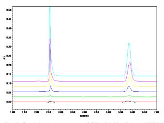
Fig.12. Overlain chromatogram of CIL (0.5-20µg/ml) and HCT (5-60 µg/ml) in mix standard
