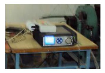
Fig 3.2 five gas analyzer
