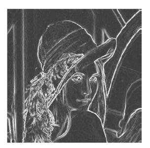
Fig.3. Detected edges by using Sobel operator
