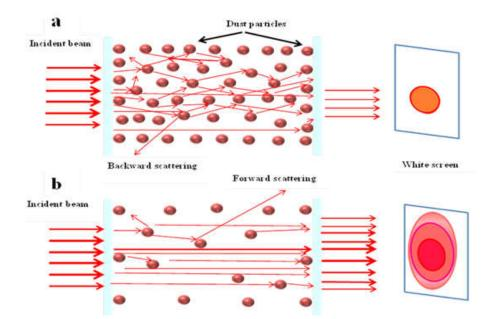
Fig. 5. Proposed model for laser scattering in dust
