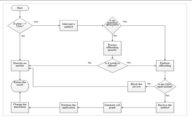
Fig 4: Execution flow of the system
