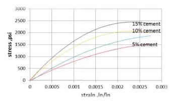
**Figure 2. Stress – strain results**
