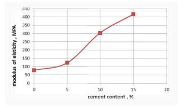
Figure 4. The modulus of elasticity
